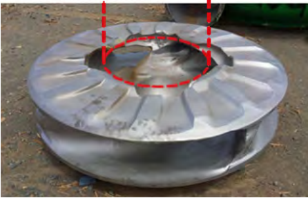
Competitor's pump impeller eye enlarged and deformed indicating suction side recirculation.
