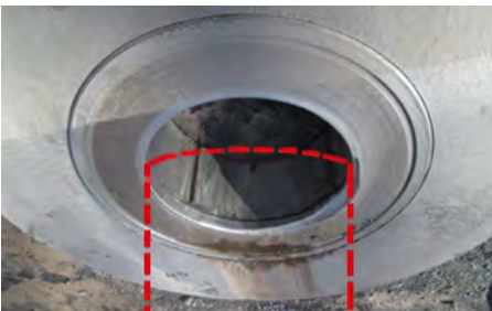
Competitor's pump impeller eye enlarged and deformed indicating suction side recirculation.
