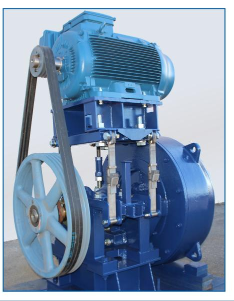
Belts can be easily re-tensioned or replaced to maximize the mount of time it takes to maintain the drive.
