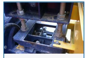
Conventional motor mounts designs are supported on four threaded rods with nuts to raise and lower the motor mount. The threads are subject to dirt and moisture and can be difficult and time consuming to move over the full length of the rod.
